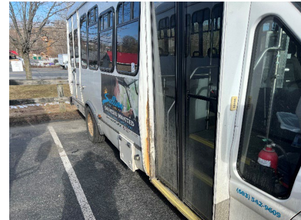
SCS: Corrosion on passenger door
