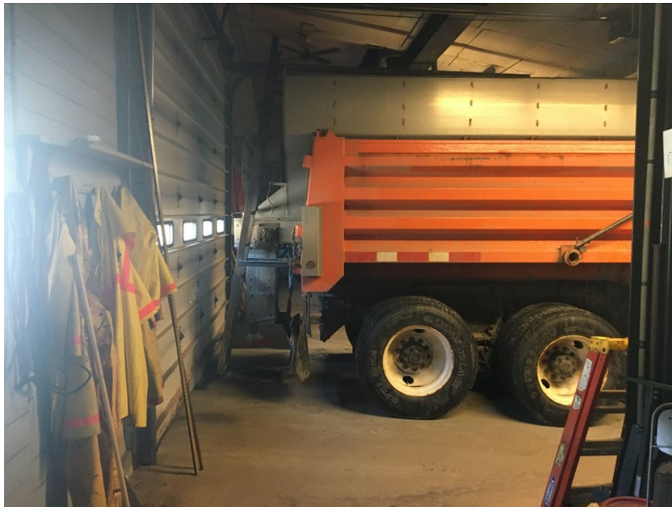
Photo-4: View of the rear of truck with plow equipment mounted and parked in shed. Overhead door barely closes behind the salt spreader.
