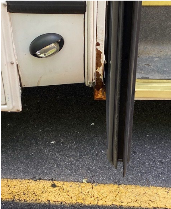
CAPSC: Corrosion on passenger door
