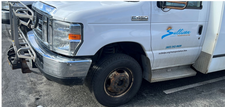
SCS: corrosion on wheel & running board
